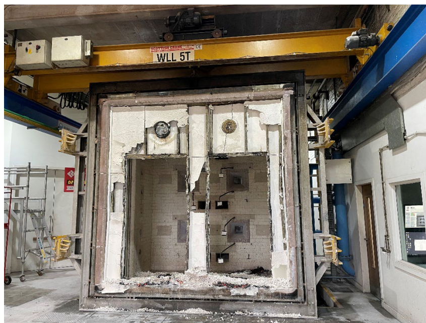
Figure 28 - The exposed surface of the test construction after the test was discontinued
