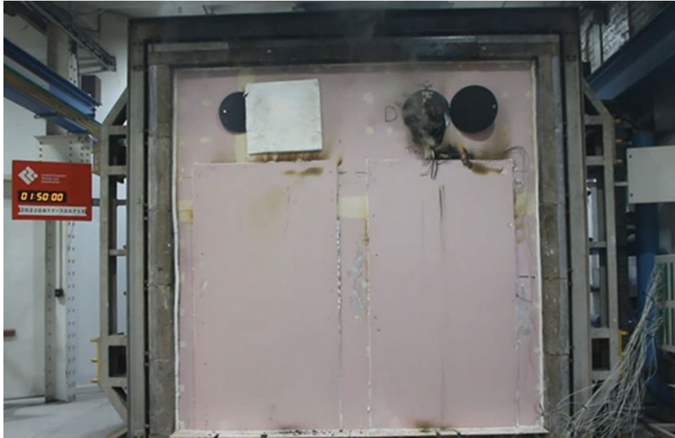
Figure 25 - The unexposed surface of the test construction after a test duration of 110 minutes
