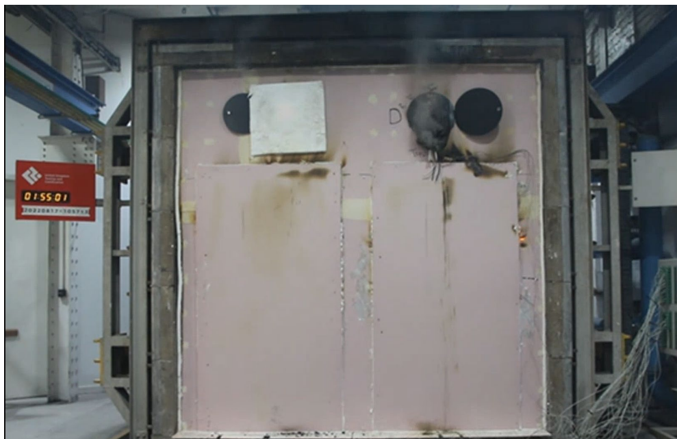
Figure 26 - The unexposed surface of the test construction after a test duration of 115 minutes
