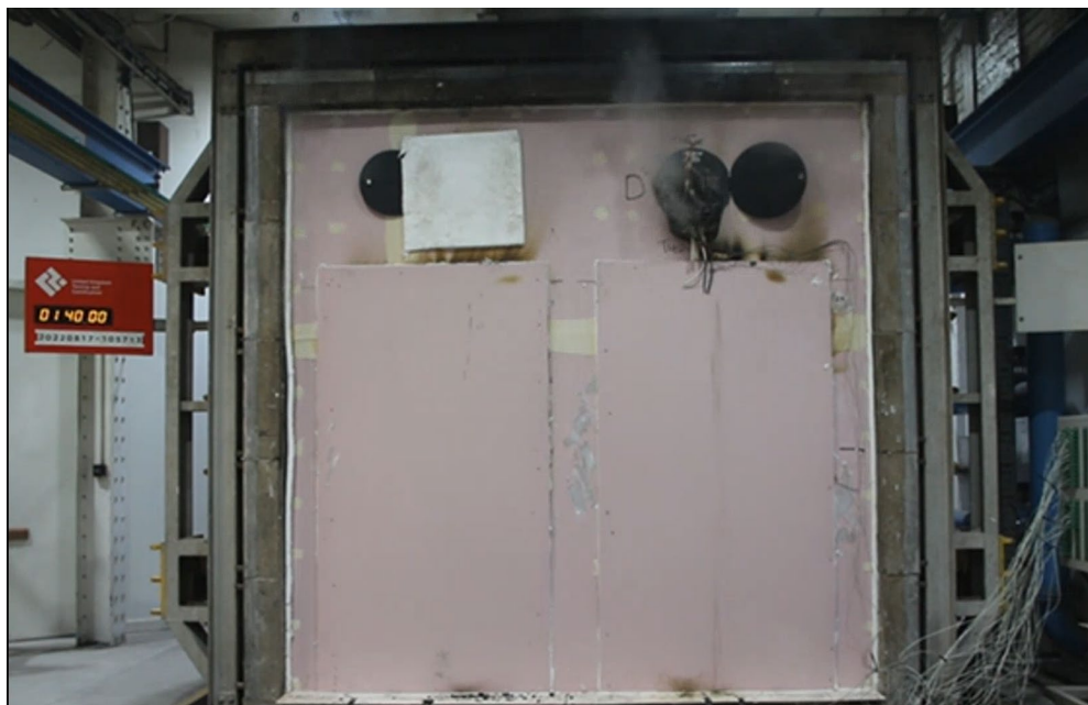
Figure 24 - The unexposed surface of the test construction after a test duration of 100 minutes
