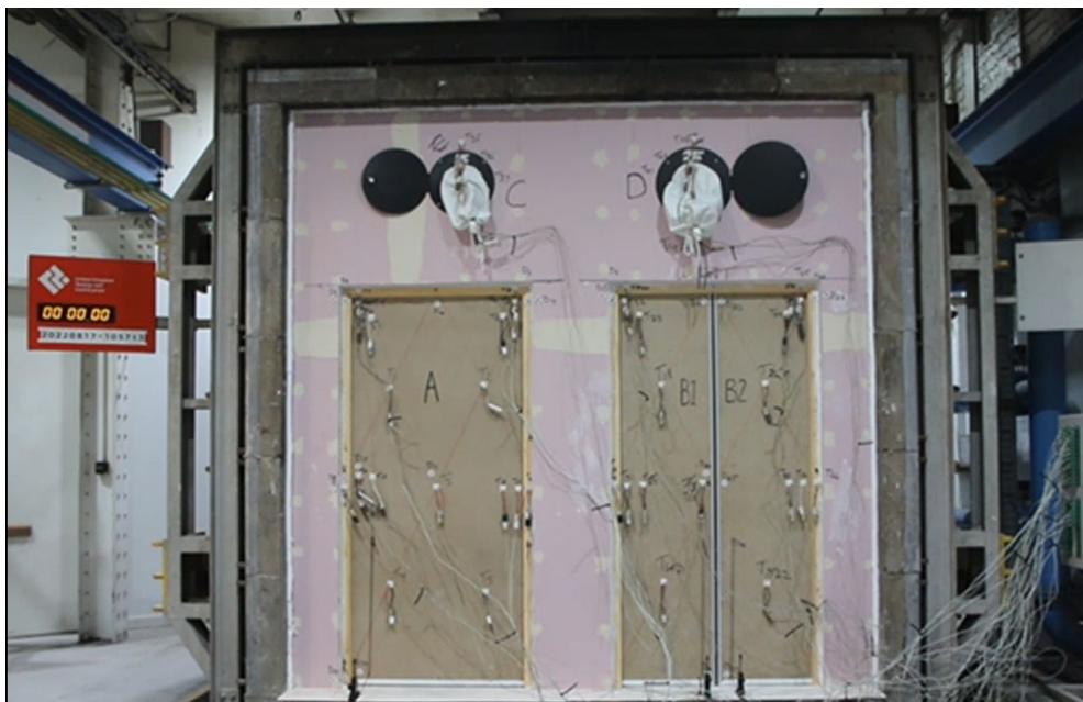
Figure 18 - The unexposed surface of the test construction prior to the commencement of the test
