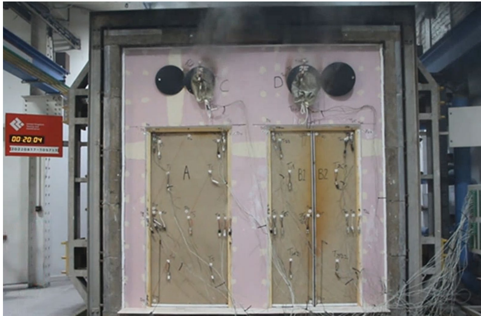
Figure 19 - The unexposed surface of the test construction after a test duration of 20 minutes
