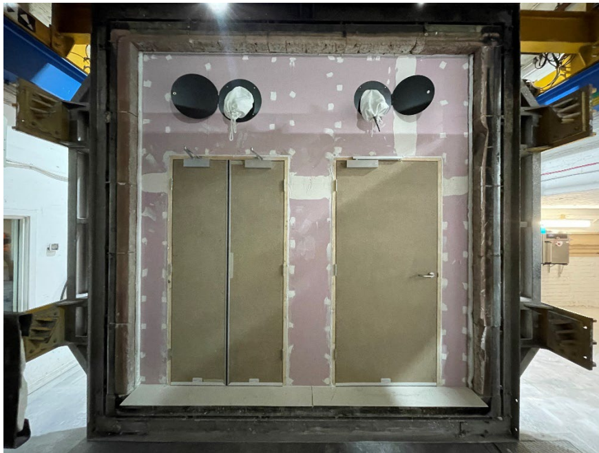
Figure 17 – The exposed surface of the test construction prior to commencement of the test
