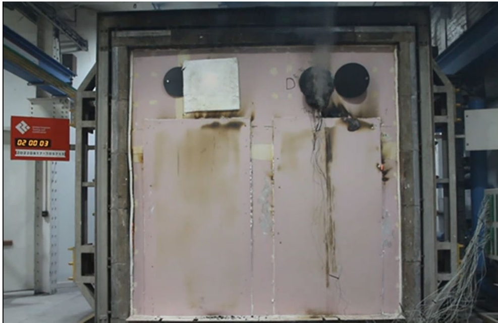
Figure 27 - The unexposed surface of the test construction after a test duration of 120 minutes
