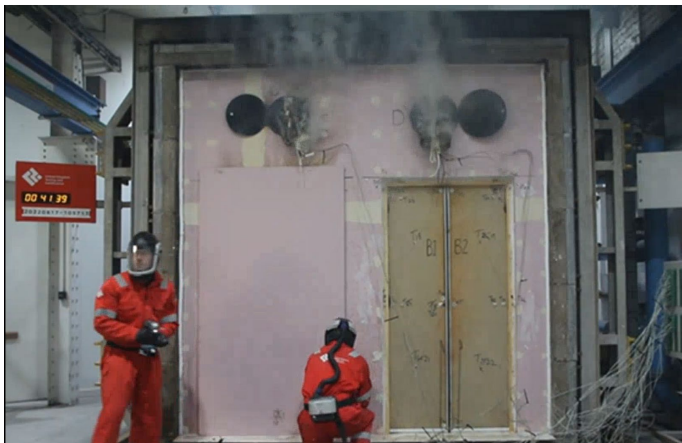
Figure 20 - The unexposed surface of the test construction after a test duration of 41 minutes
