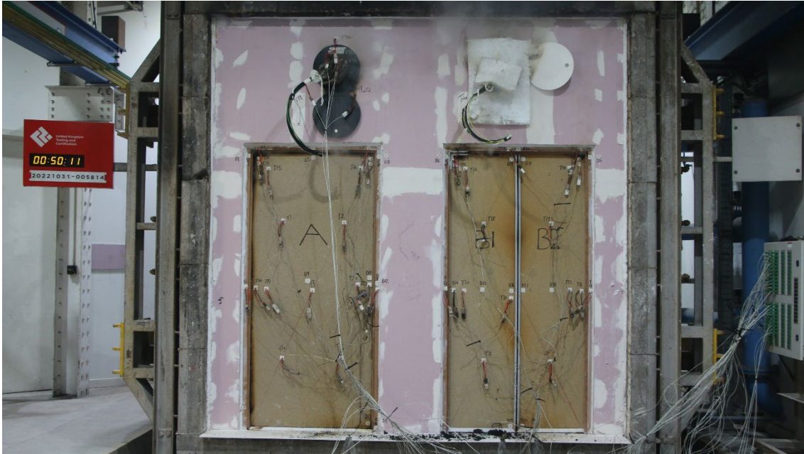
Figure 26 - The unexposed surface of the test construction after a test duration of 50 minutes
