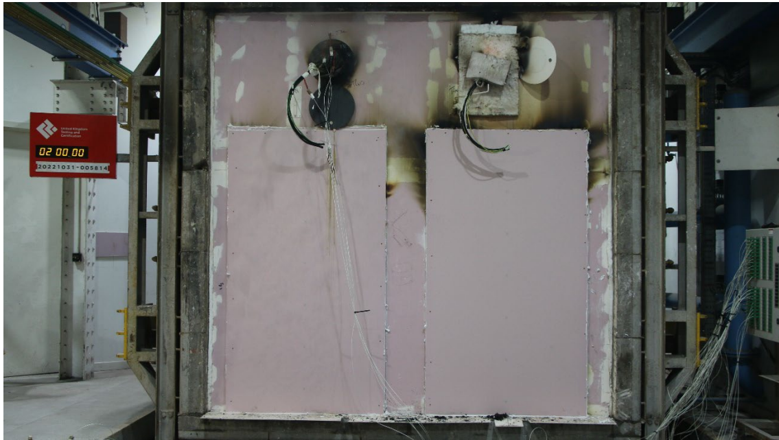
Figure 32 - The unexposed surface of the test construction after a test duration of 120 minutes
