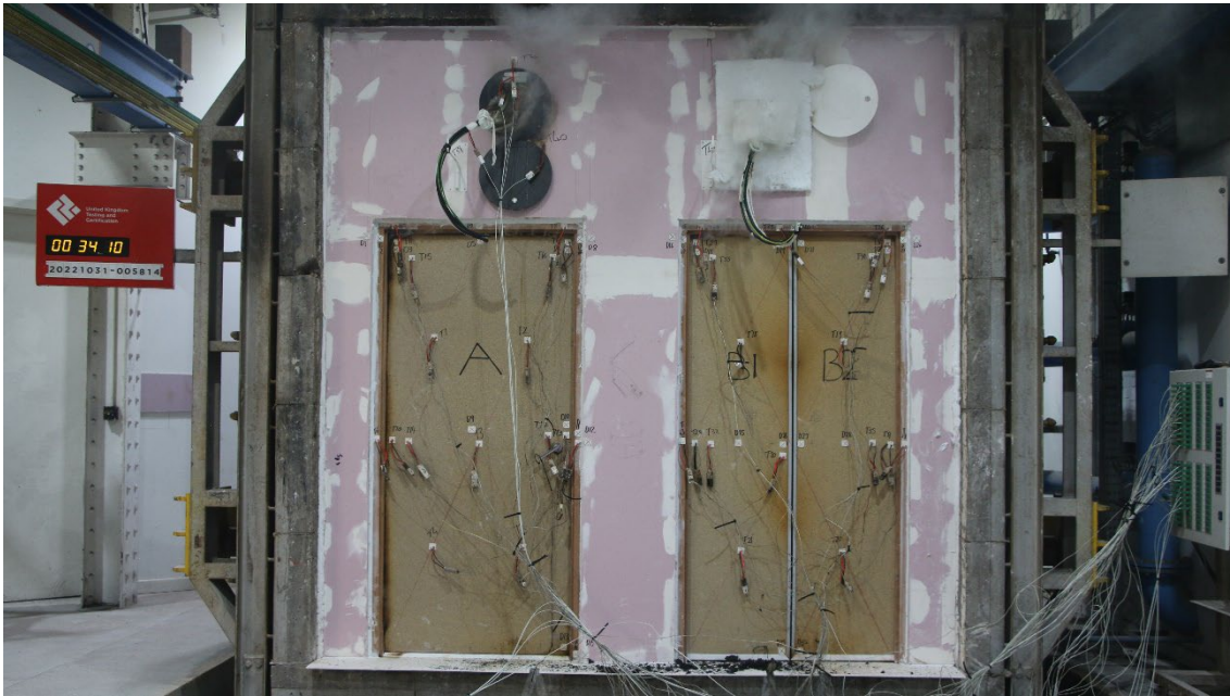
Figure 24 - The unexposed surface of the test construction after a test duration of 34 minutes
