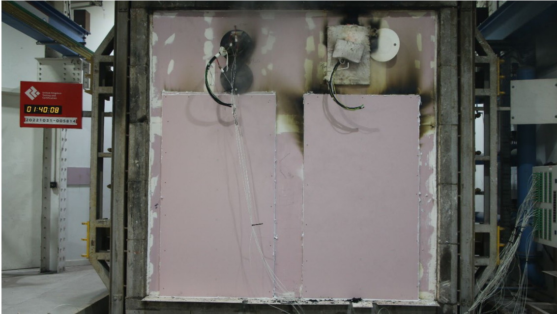
Figure 30 - The unexposed surface of the test construction after a test duration of 100 minutes
