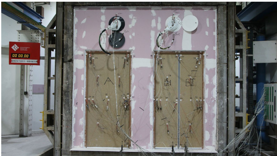
Figure 21 - The unexposed surface of the test construction prior to the commencement of the test
