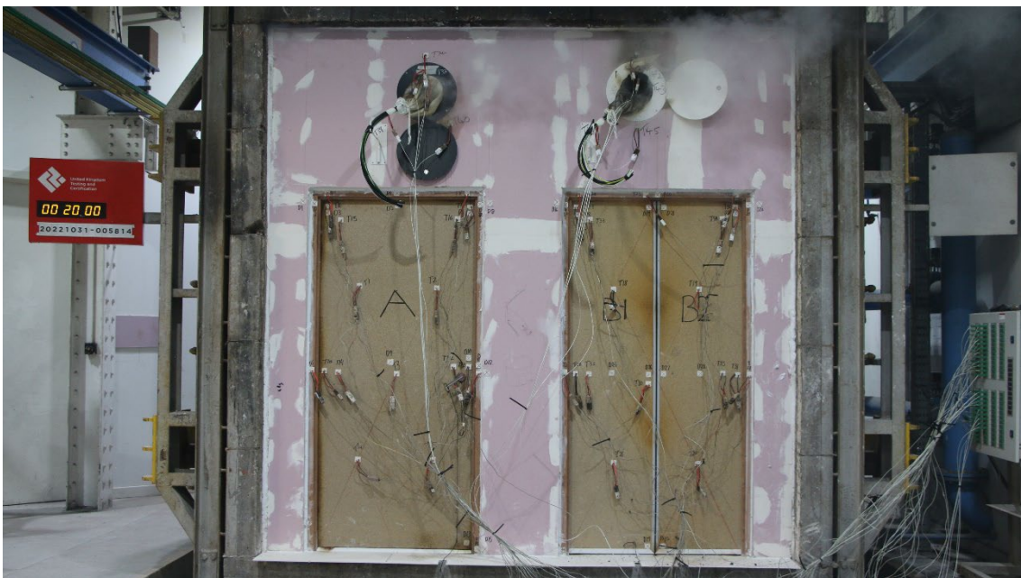
Figure 23 - The unexposed surface of the test construction after a test duration of 20 minutes
