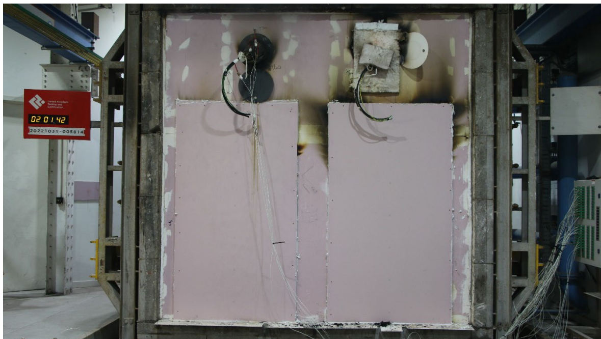
Figure 33 - The unexposed surface of the test construction after a test duration of 121 minutes
