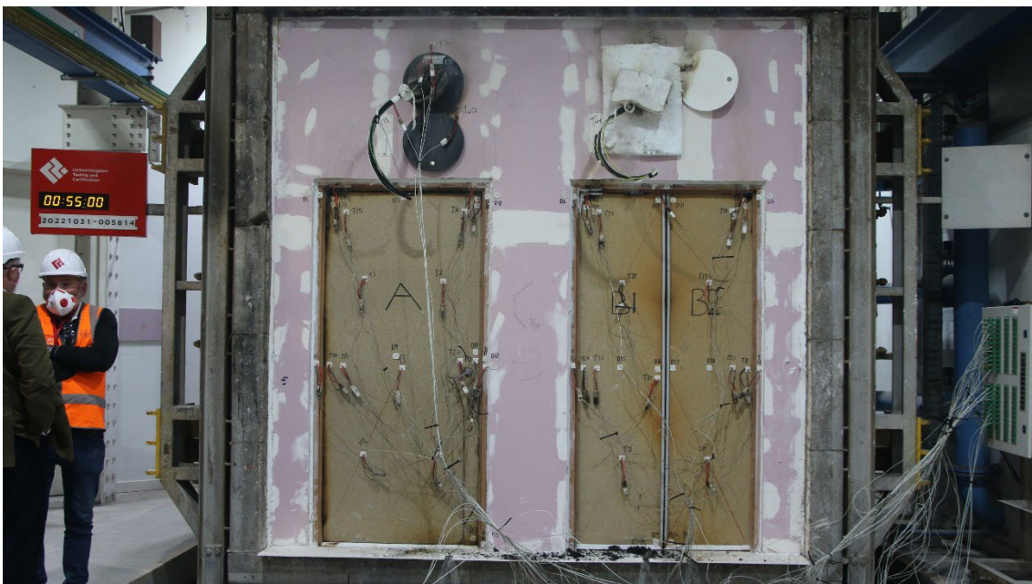
Figure 27 - The unexposed surface of the test construction after a test duration of 55 minutes
