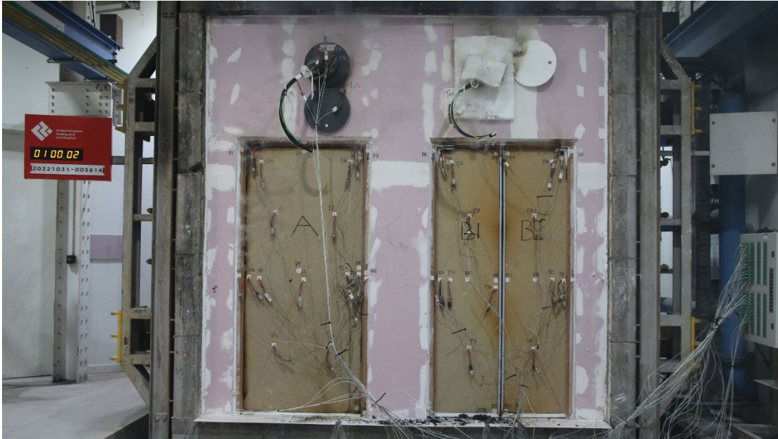
Figure 28 - The unexposed surface of the test construction after a test duration of 60 minutes
