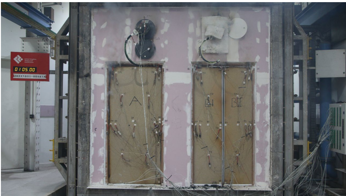
Figure 29 - The unexposed surface of the test construction after a test duration of 65 minutes
