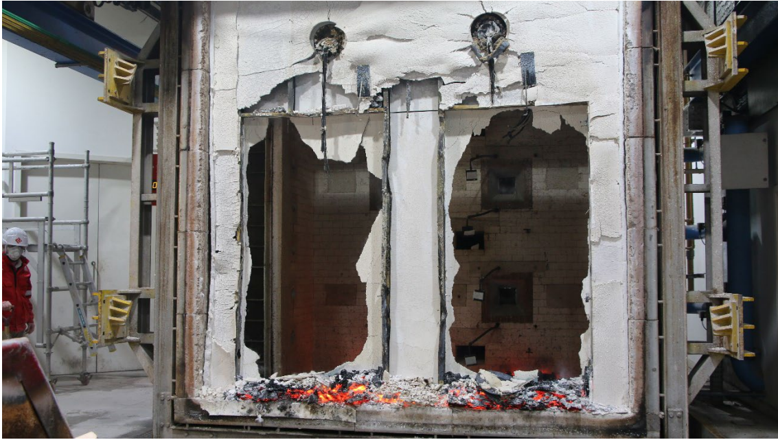
Figure 34 - The exposed surface of the test construction after the test was discontinued
