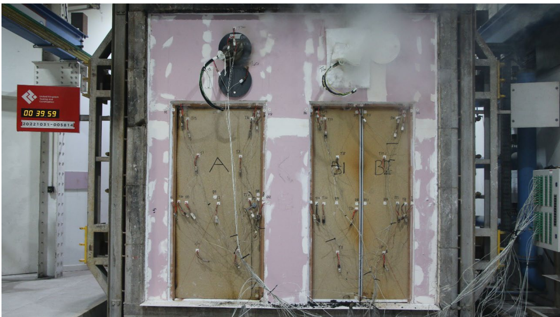
Figure 25 - The unexposed surface of the test construction after a test duration of 39 minutes
