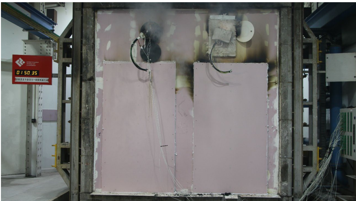
Figure 31 - The unexposed surface of the test construction after a test duration of 110 minutes
