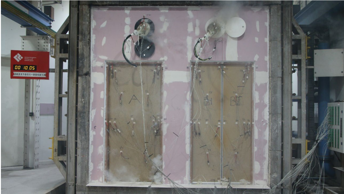
Figure 22 - The unexposed surface of the test construction after a test duration of 10 minutes
