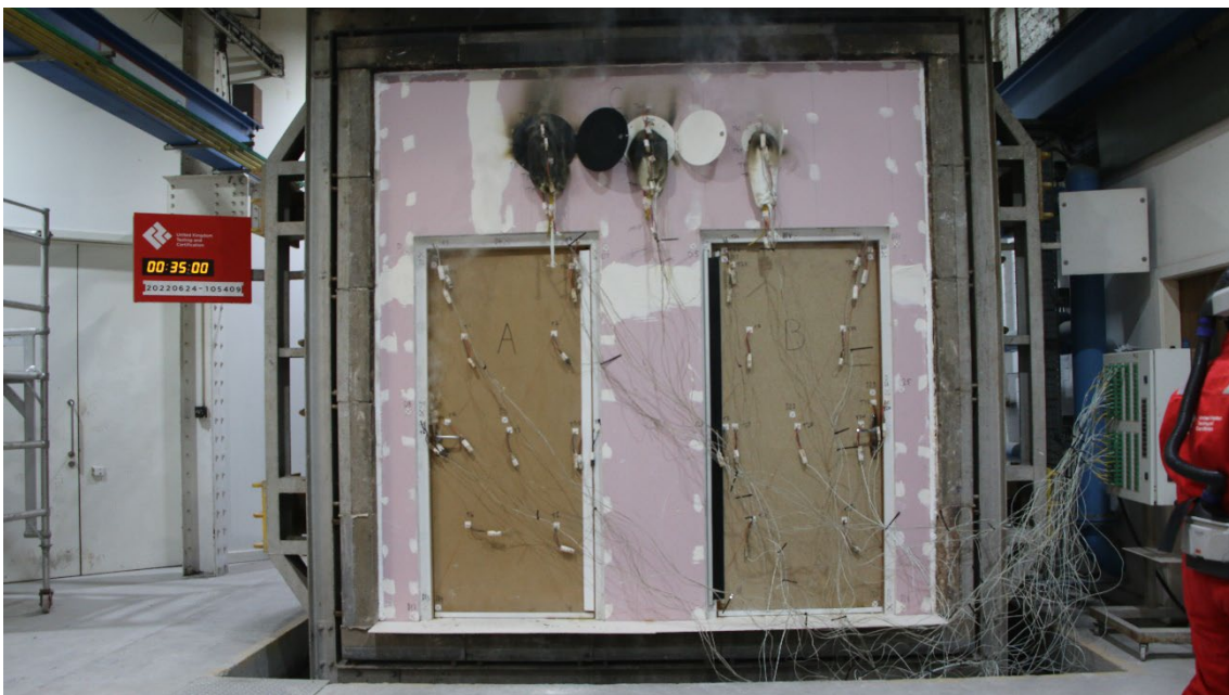
Figure 22 - The unexposed surface of the test construction after a test duration of 35 minutes
