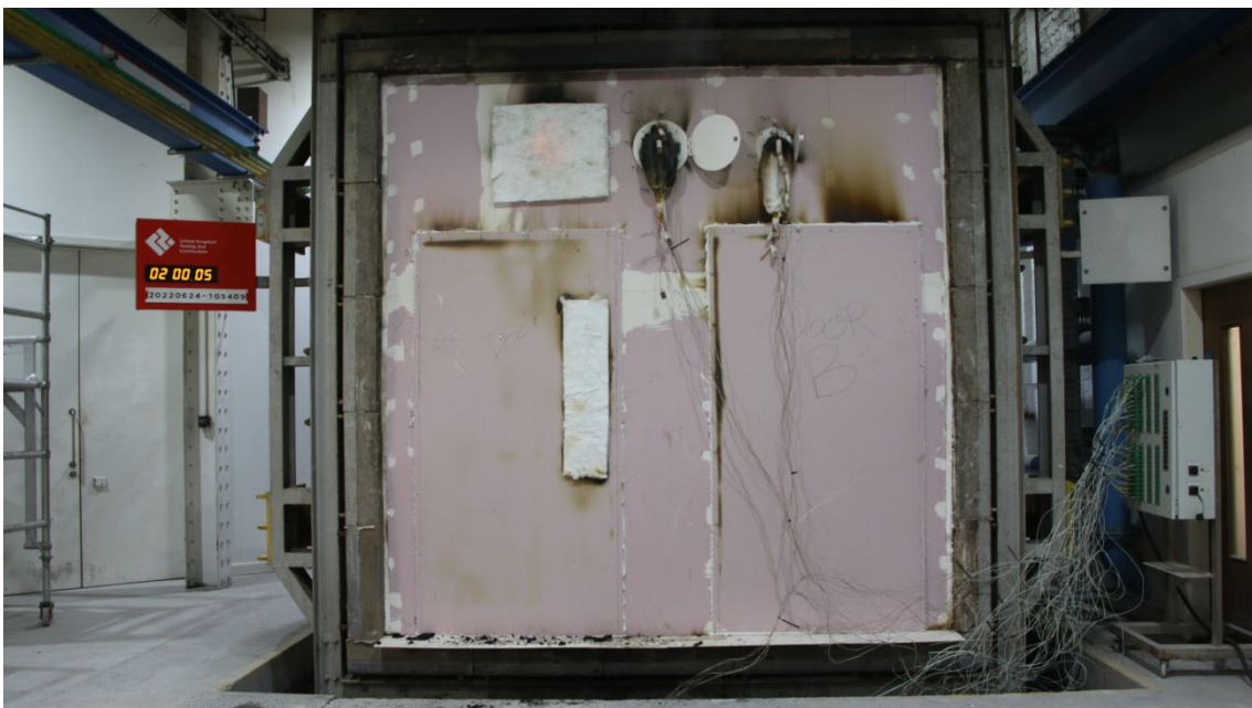
Figure 30 - The unexposed surface of the test construction after a test duration of 120 minutes
