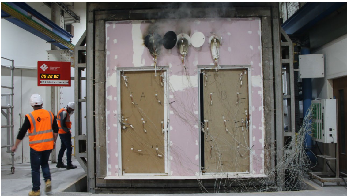
Figure 20 - The unexposed surface of the test construction after a test duration of 20 minutes
