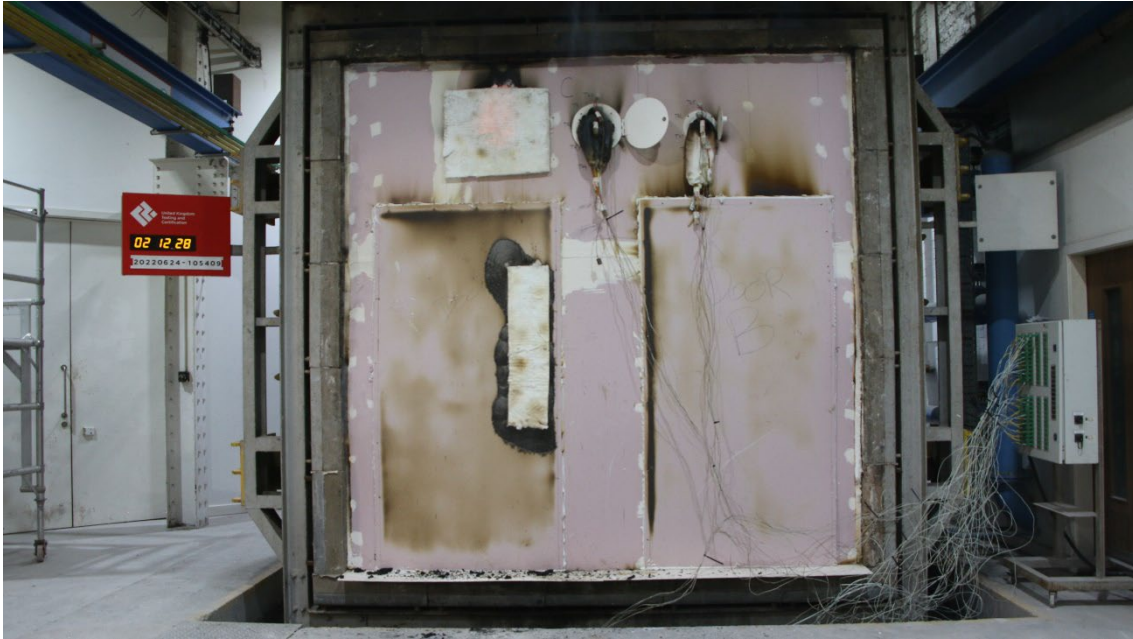
Figure 31 - The unexposed surface of the test construction after a test duration of 132 minutes
