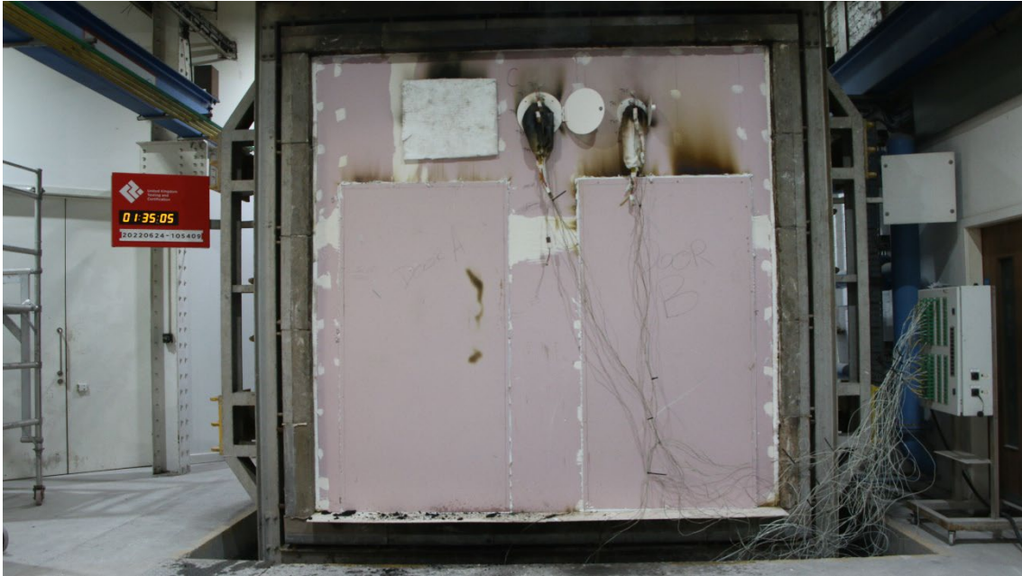
Figure 27 - The unexposed surface of the test construction after a test duration of 95 minutes
