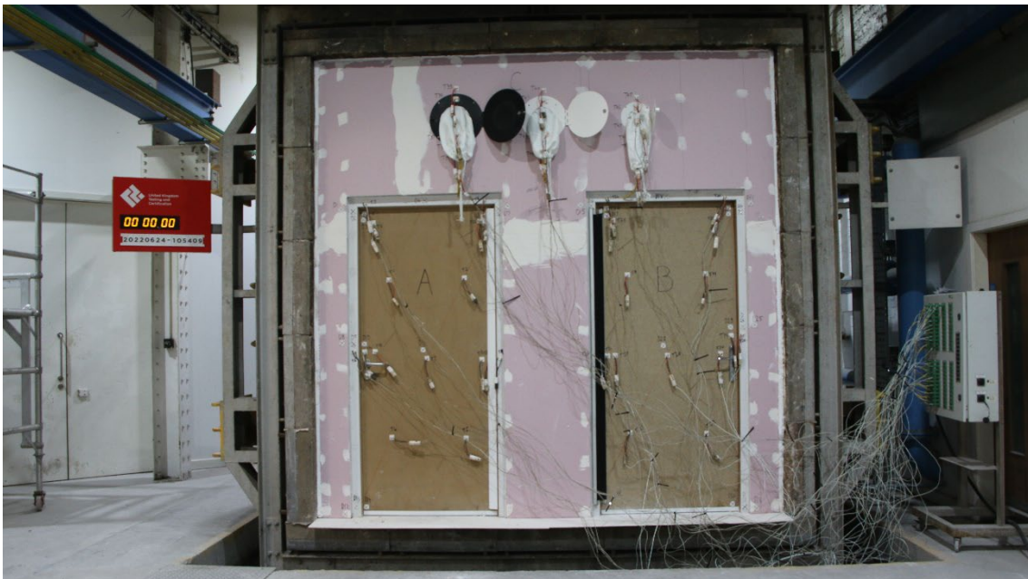
Figure 18 - The unexposed surface of the test construction prior to the commencement of the test
