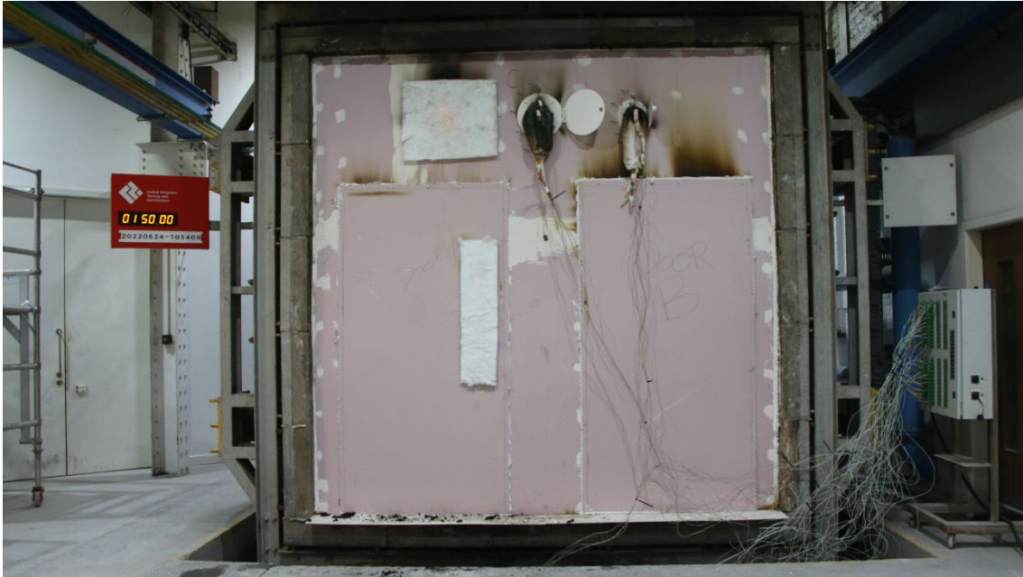
Figure 29 - The unexposed surface of the test construction after a test duration of 110 minutes
